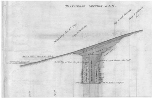
Figure 2 - Section showing the repairs to the arm trench in 1882
